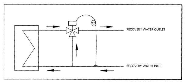
In this way, water flow will increase in proportion to the increase in water temperature, thereby ensuring optimal unit operation (see figure on next page).
